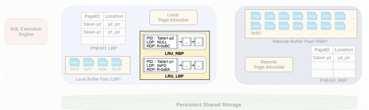
Two-level LRU : hold all metadata of local and remote pages, reduce communications with remote memory node
