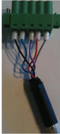
Figure 11.2: Wiring scheme from above: black, blue, purple, red, grey
