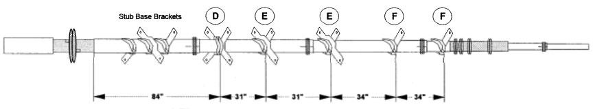
NOTE: All measurements measured to the TOP of each insulator
