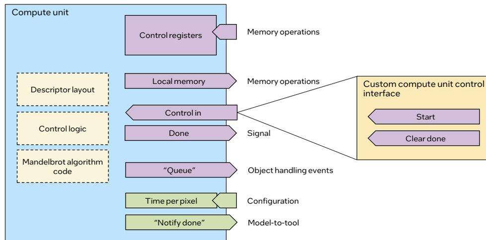
The external interface of the compute unit contains the following:
