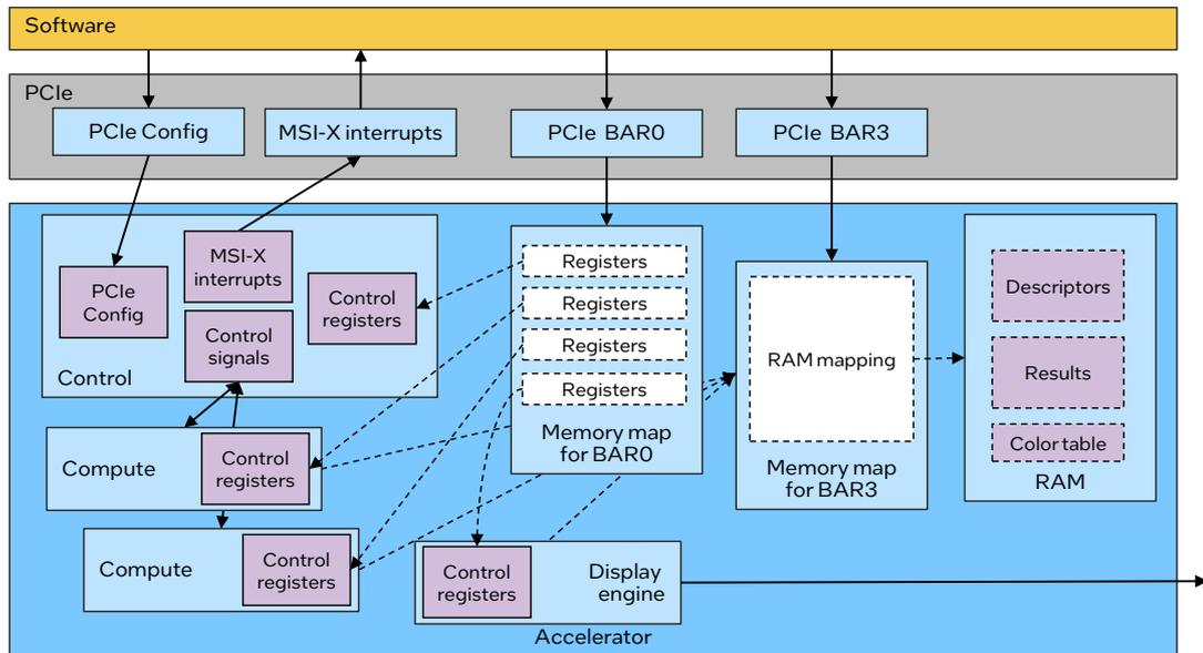
The **control unit** contains the main control registers for the accelerator, as well as the PCIe interface. It manages computation jobs in the compute units via a set of signals to and from the compute units.
